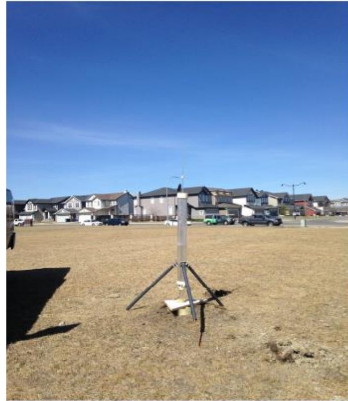
Photo 2. View of Permeameter testing at subject site.
