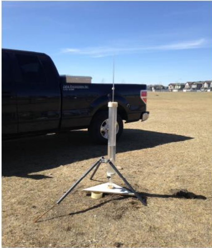
Photo 1. View of Permeameter testing at subject site.
